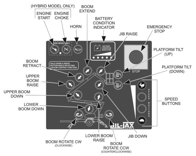
Figure 3-2. Platform Control Station
